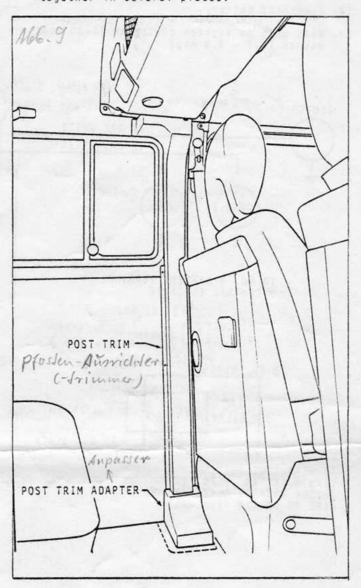
26- Install post trim and post trim adapter with #6 x 1/2" black sms and black flatwashers. Screws for post trim should be secured to braces behind trim panel.
