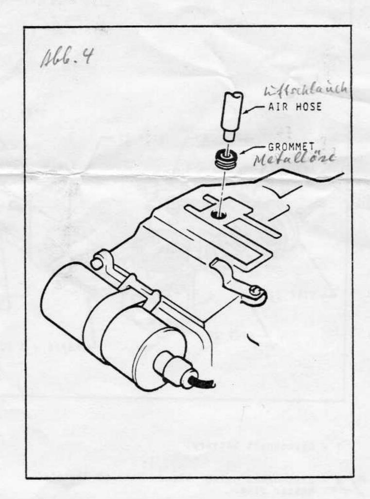
35- Drill 3/4" dia. hole in fan housing sheetmetal. Install grommet. Remove elbow from air hose (removed in step 4) and plug it in.
