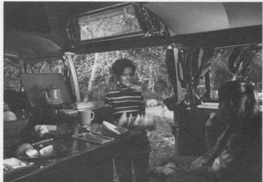
Besides providing plenty of extra storage space, the Adventurer top provides 6' of standing room, 2 large, screened, awning-style windows (they can be left open on rainy days), a wind-adjusted roof vent with built-in 12 V reversible fan and 2 extra interior lights.
