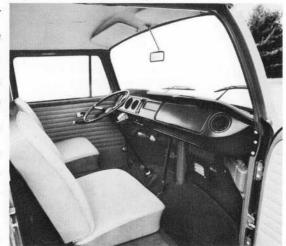
include a 9-position driver's seat, a padded dashboard with recessed dials, a fresh air ventilating system, a 2-speed wiper knob, a pneumatic windshield washer system plus many other VW touches.
